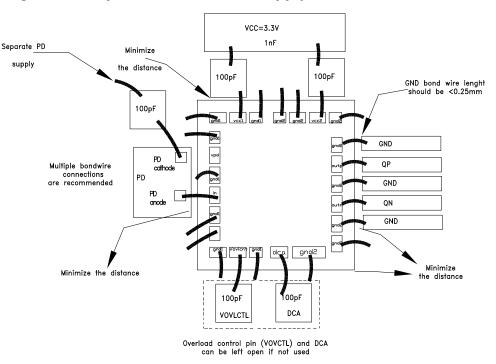
Suggested assembly configuration for separate photo diode supply. Suggested bond-wire length for optimum performance is as follows:
