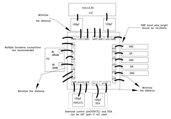
Suggested assembly configuration for using internal supply for photo-diode. Suggested bond-wire length for optimum performance is as follows:
