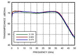
[1] 50  $\Omega$  on wafer measurement results . [2] Assumes photo diode and assembly model on page 3.
