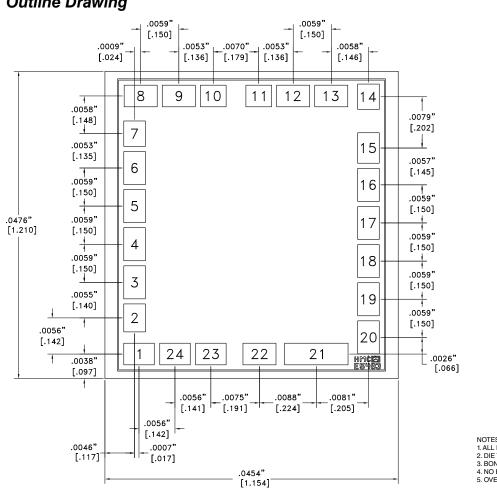
NOTES: 1. ALL DIMENSIONS ARE IN INCHES [MM] 2. DIE THICKNESS IS .006" 3. BOND PAD METALIZATION: ALUMINUM 4. NO BACKSIDE METAL 5. OVERALL DIE SIZE ±.002'
