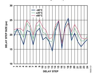
Figure 22. Analog Delay Step Size vs Delay Step over Temperature, LVPECL at 3072 MHz with Digital Delay = 1
