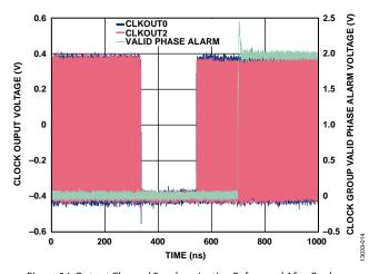
Figure 24. Output Channel Synchronization Before and After Rephase
