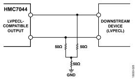
Figure 32. DC-Coupled LVPECL Output Driver
