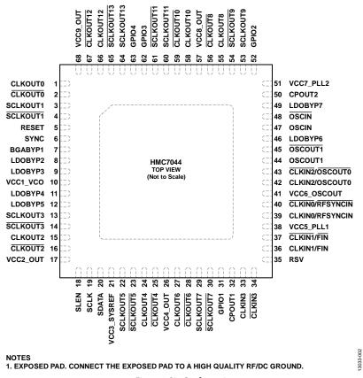
Figure 2. Pin Configuration
