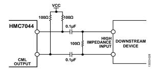
Figure 28. AC-Coupled CML (Configured High-Z) Output Driver
