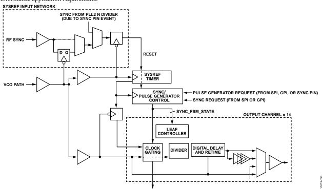
Figure 44. Clock Output Network Simplified Diagram
