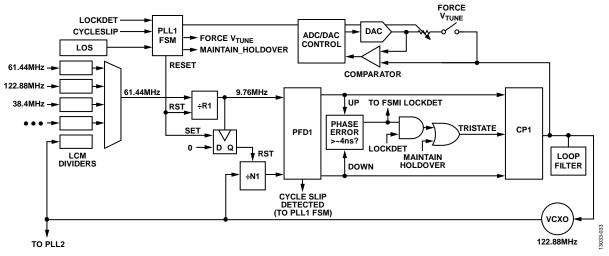
Figure 36. PLL1 Architecture with a Typical Frequency Configuration
