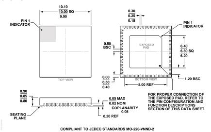
Figure 54. 68-Lead Lead Frame Chip Scale Package [LFCSP\_VQ] 10 mm × 10 mm Body, Very Thin Quad (HCP-68-1)
