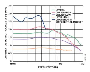
Figure 13. Differential Output Voltage vs. Frequency at Different Modes
