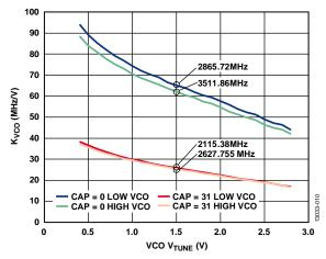
Figure 11. VCO Gain (K<sub>VCO</sub>) vs. VCO V<sub>TUNE</sub>
