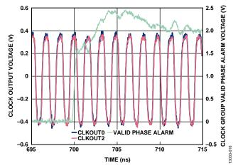
Figure 26. Output Channel Synchronization After Rephase
