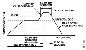
Figure 51. Pb-Free Reflow Solder Profile
