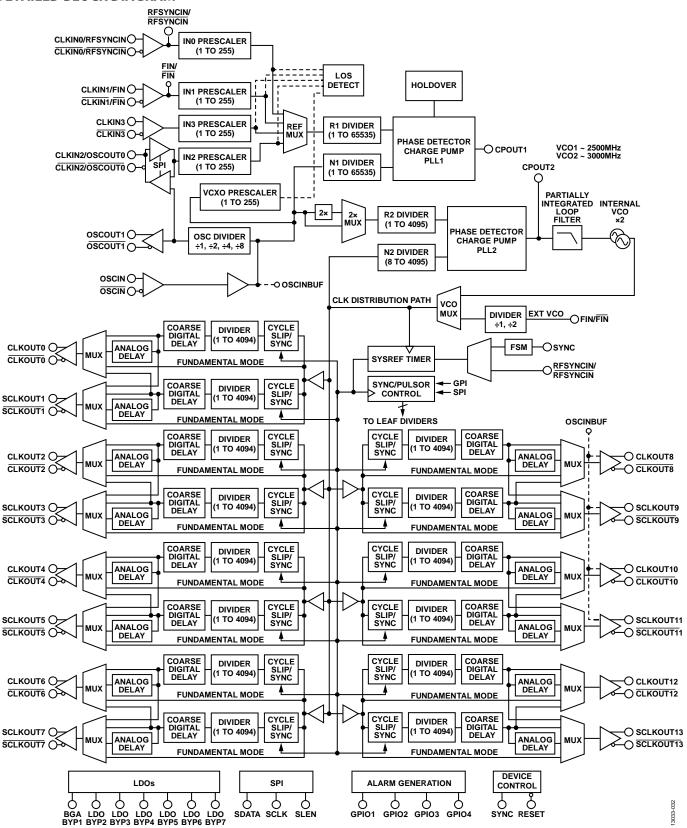
Figure 35. Top Level Diagram
