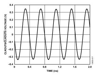
Figure 16. Differential CLKOUTO/CLKOUTO at 2457 MHz, LVPECL
