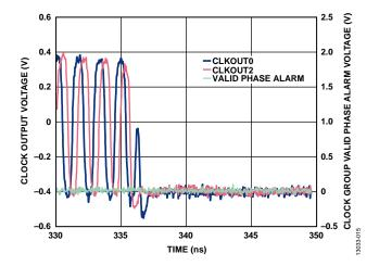
Figure 25. Output Channel Synchronization Before Rephase
