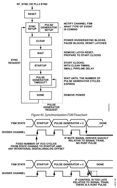
Figure 46. Start-Up Behavior of an Example Divider Configured as a Pulse Generator
