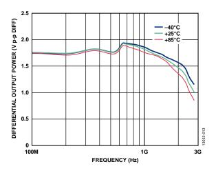
Figure 15. LVPECL Differential Output Voltage vs. Frequency at Different Temperatures
