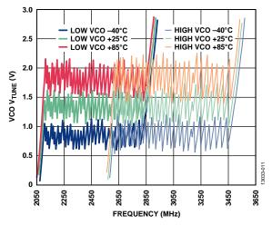
Figure 12. VCO V<sub>TUNE</sub> vs. Frequency
