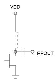
FIGURE 6.  $\ensuremath{\mathsf{VDD}}$  and RFout interface schematic.
