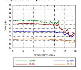
[1] VR = 0.0 V [2] Frequency = 13 GHz [3] Vee = -3.3 V [4] Device measured on evaluation board with gating after connector
