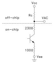
The value of the resistor can be chosen using the following equation as a function of VAC. VAC DC voltage value can be chosen by using the plot given above.
