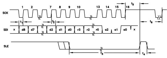
Figure 10. SPI Timing Diagram, Write Operation
