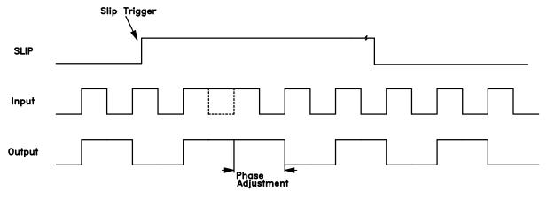
Figure 3. HMC988LP3E's SLIP Function Timing Diagram
