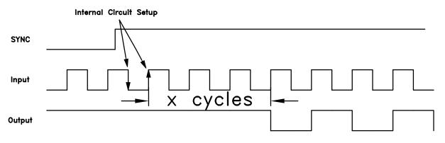
Figure 2. HMC988LP3E SYNC Function Timing Diagram
