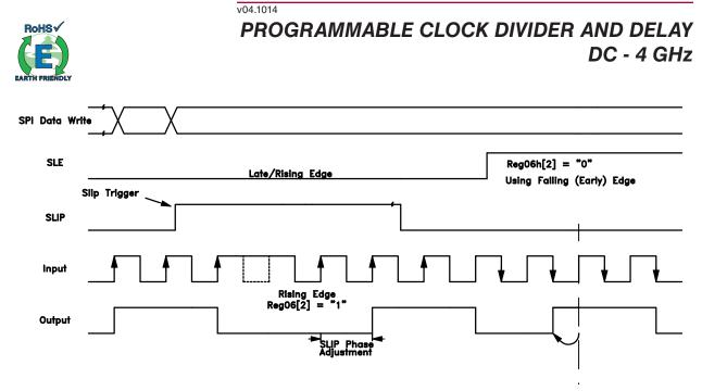
Figure 4. Delay by 1/2 of Input Clock Cycle Timing Diagram
