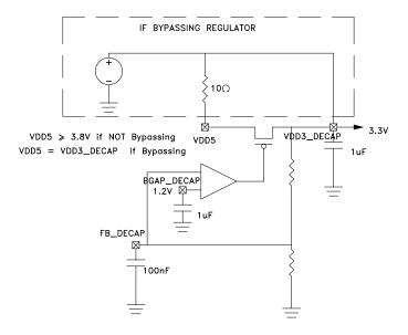
Figure 6. Regulator Circuit Diagram
