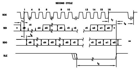
Figure 11. SPI Diagram, Read Operation 2- Cycles
