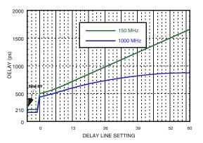
[1] Measured Differential input and out at various frequencies. Under 300 MHz, the measurment is restricted by the instrument. [2]Measured single-ended. 120 Ω DC termination, 3.3 V 1 +6 dBm single-ended input. HMC988LP3E AC coupled to 50 Ω instrument with divider bypass
