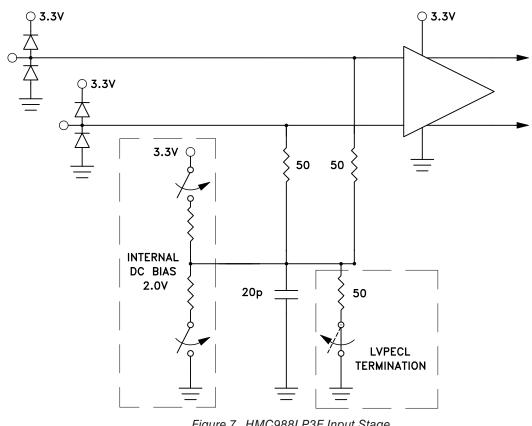
Figure 7. HMC988LP3E Input Stage
