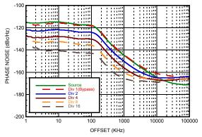
Figure 3. Phase Noise Floor Performance Vs Input Swing
