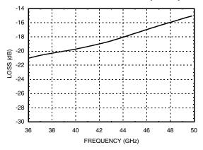
Return Loss vs. Frequency @ Minimum Attenuation
