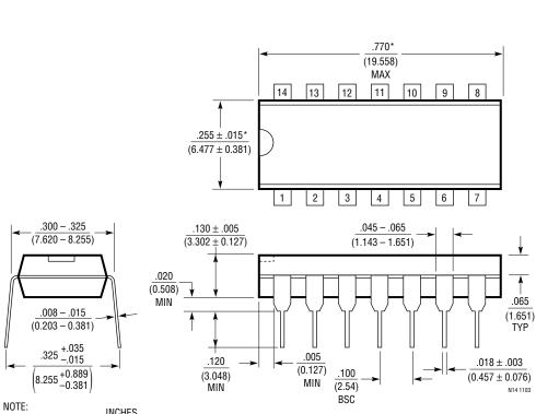
N Package 14-Lead PDIP (Narrow .300 Inch) (Reference LTC DWG # 05-08-1510)
