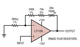
Gain 1000 Amplifier with 0.01% Accuracy, DC to 5Hz
