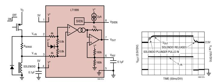
Figure 8. Solenoid Current Monitor for Ground Tied Solenoid. The Common Mode Inputs to the LT1999 Switch Between  $\mathbf{V}_S$  and One Diode Drop Below Ground
