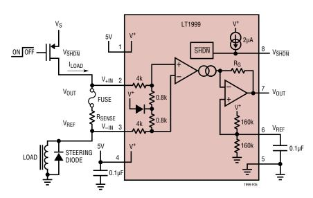
Figure 6. Using the LT1999 to Monitor a Fuse
