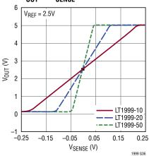
$\mbox{V}_{\mbox{\scriptsize OUT}}$  vs  $\mbox{V}_{\mbox{\scriptsize SENSE}}$  Over the Sense ABSMAX Range
