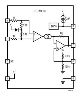
Figure 1. Simplified Block Diagram
