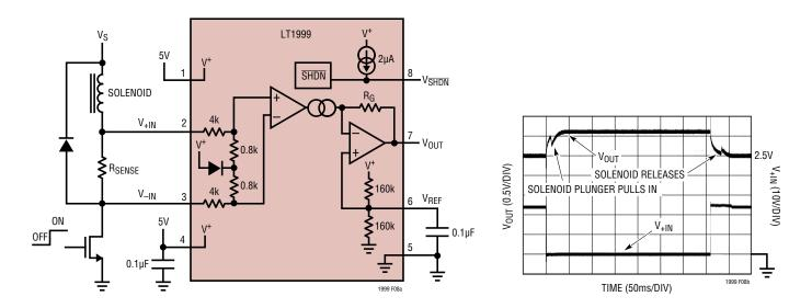
Figure 9. Solenoid Current Monitor for Non-Grounded Solenoids. This Circuit Performs the Same Function as Figure 7 Except One End of the Solenoid Is Tied to  $V_S$ . The Common Mode Voltage of Inputs of the LT1999 Switch Between Ground and One Diode Drop Above  $V_S$
