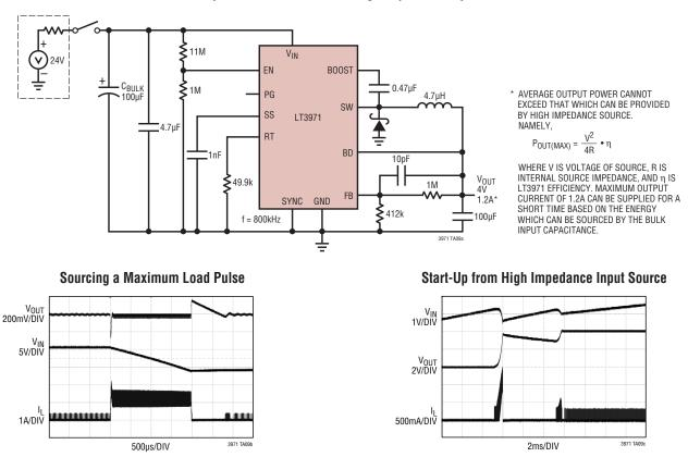
4V Step-Down Converter with a High Impedance Input Source
