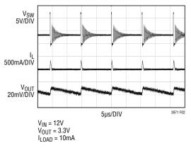
Figure 2. Burst Mode Operation
