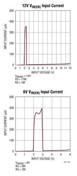
Figure 6. Input Current vs Input Voltage for a Programmed  $V_{\text{IN}(\text{EN})}$  of 6V and 12V
