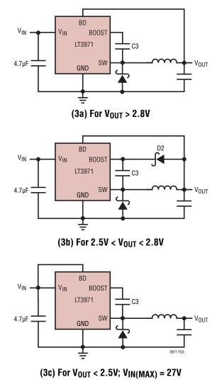
Figure 3. Three Circuits for Generating the Boost Voltage
