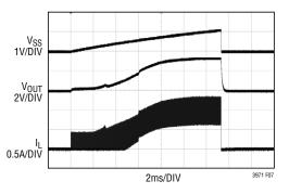
Figure 7. Soft-Start Waveforms for Front-Page Application with 10nF Capacitor on SS. EN is Pulsed High for About 13ms with a  $3.3\Omega$  Load Resistor
