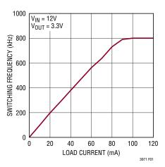
Figure 1. Switching Frequency in Burst Mode Operation
