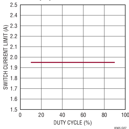
Switch Current Limit vs Duty Cycle
