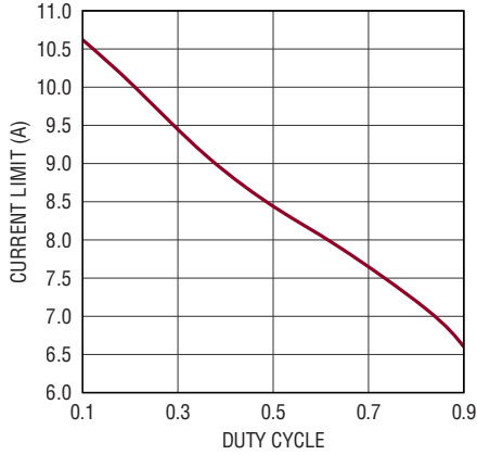
Top FET Current Limit vs Duty Cycle
