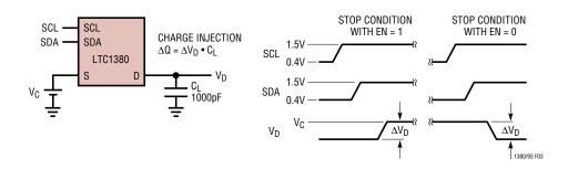
Figure 3. Charge Injection Test
