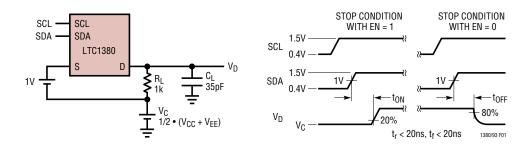
Figure 1. Switch  $t_{\text{ON}}/t_{\text{OFF}}$  Propagation Delay from SMBus STOP Condition
