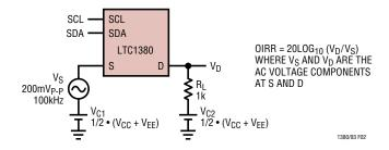
Figure 2. Off-Channel Isolation (OIRR) Test
