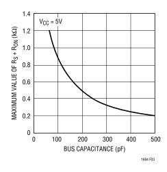
Figure 3. Maximum Value of  $R_S + R_{ON}$  as a Function of Bus Capacitance for Meeting the SMBus  $t_{f(MAX)}$  Requirement
