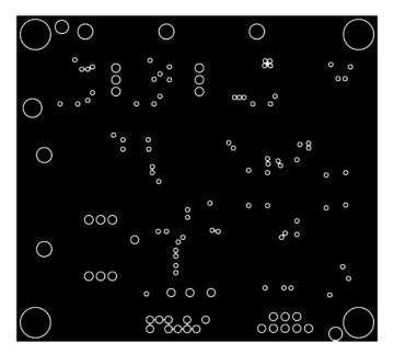
Figure 18. Layer 2 GND Plane
