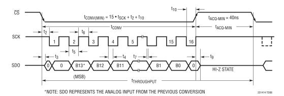
Figure 6: LTC2314-14 Serial Interface Timing Diagram (SCK High During t<sub>ACO</sub>)
