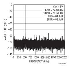
Figure 13. 32k Point FFT of the LTC2314-14 at  $f_{\text{IN}}$  = 500 kHz
