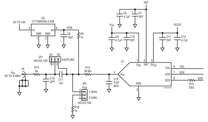
Figure 21. Partial 1563 Demo Board Schematic
