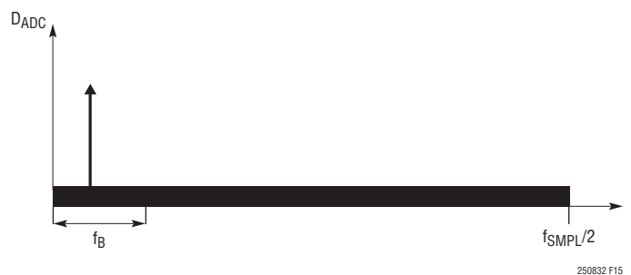
Figure 15. Frequency Spectrum of SAR ADC Core Output
