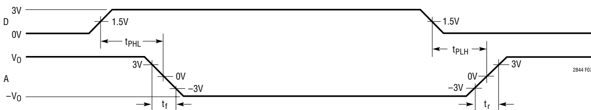
Figure 7. V.10, V.28 Driver Propagation Delays
