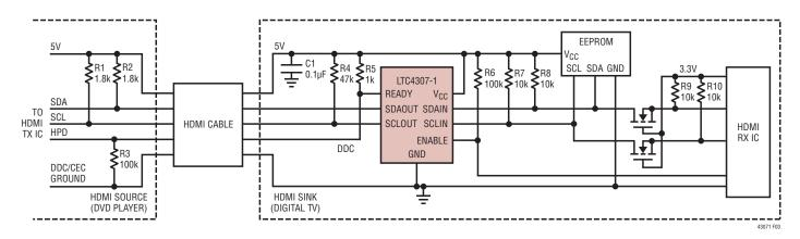
Figure 3. The LTC4307-1 in HDMI Capacitance Buffering Application
