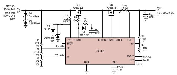
Figure 1. 4A, 12V Overvoltage Output Regulator with Reverse Current Protection
