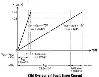
Figure 3. Fault Timer Current of the LTC4364
