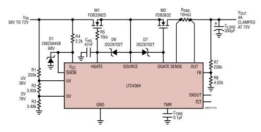
Figure 10. 48V Hot Swap with Overvoltage Output Regulation at 72V, Circuit Breaker, and Reverse Current Protection
