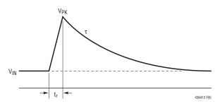
Figure 5. Prototypical Transient Waveform
