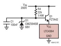
Figure 7. Buffering V<sub>CC</sub> to Extend Input Supply Range
