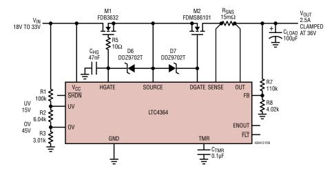
Figure 9. 28V Hot Swap with Overvoltage Output Regulation at 27V, Circuit Breaker, and Reverse Current Protection
