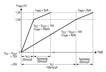
(3a) Overvoltage Fault Timer Current
