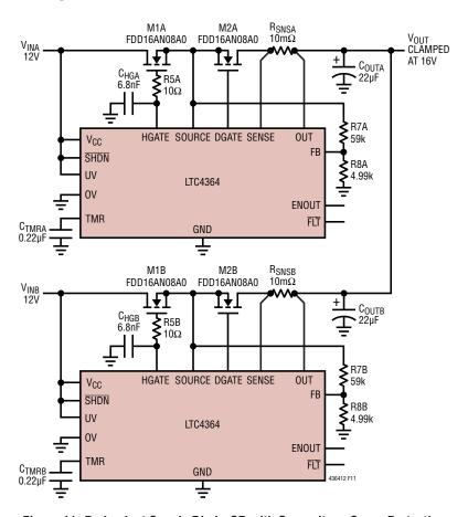
Figure 11. Redundant Supply Diode-OR with Overvoltage Surge Protection
