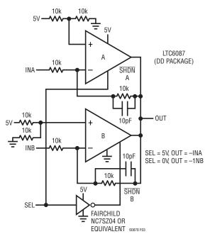
Figure 3. Inverting Amplifier with Muxed Output
