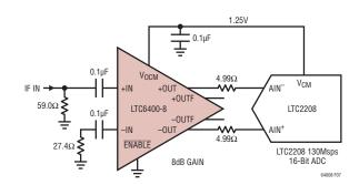
Figure 7. Single-Ended Input to LTC6400-8 and LTC2208
