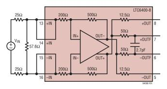
Figure 1. Input Termination for Differential  $50\Omega$  Input Impedance Using Shunt Resistor
