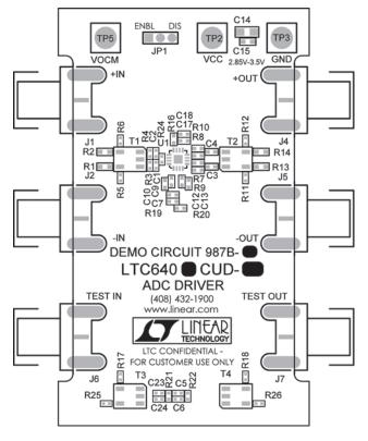
Figure 9. Top Silkscreen for DC987B. Test Circuit A
