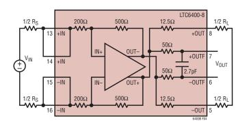
Figure 4. Calculate Differential Gain
