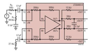
Figure 3. Input Termination for Single-Ended  $50\Omega$  Input Impedance
