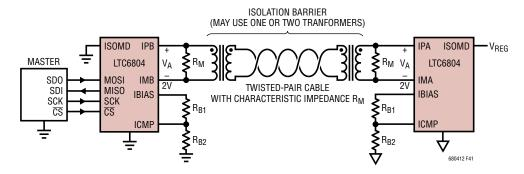
Figure 41. isoSPI Circuit
