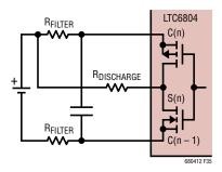
Figure 35. Internal Discharge Circuit
