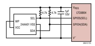
Figure 25. Connecting I<sup>2</sup>C EEPROM to LTC6804 GPIO Pins
