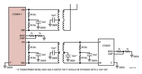
Figure 46. Interfacing an LTC6804-1 with a µC Using an LTC6820 for Isolated SPI Control
