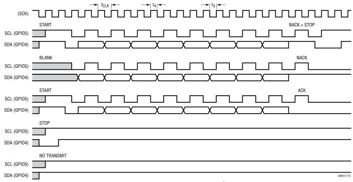
Figure 12. STCOMM Timing Diagram for an I<sup>2</sup>C Master
