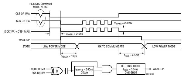
Figure 21. Wake-Up Detection and IDLE Timer
