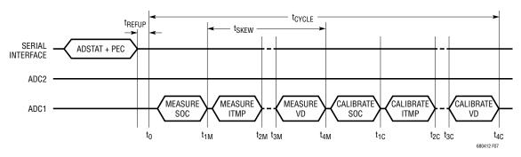
Figure 7. Timing for ADSTAT Command Measuring SOC, ITMP, VA, VD
