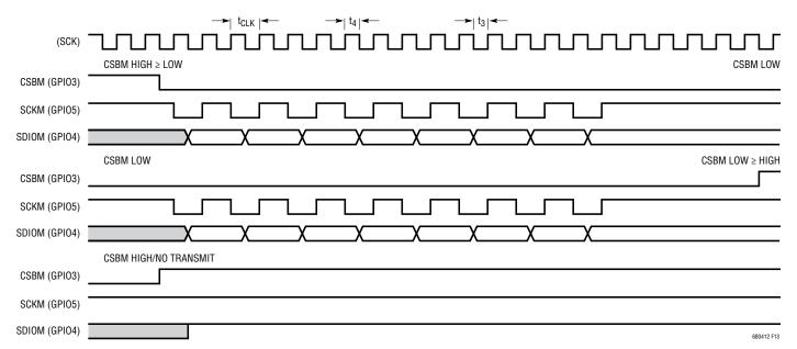
Figure 13. STCOMM Timing Diagram for a SPI Master
