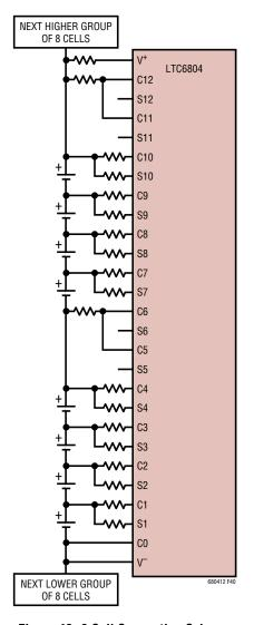
Figure 40. 8 Cell Connection Scheme
