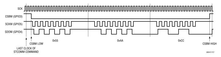
Figure 27. LTC6804 SPI Communication Example
