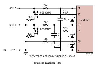
Figure 34. Input Filter Structure Configurations
