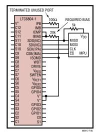
Figure 18c. Single-Device LTC6804-1 Using 4-Wire Port A
