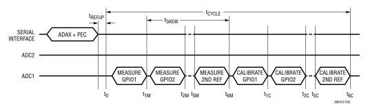
Figure 5. Timing for ADAX Command Measuring All GPIOs and 2nd Reference
