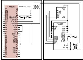
Figure 18a. Single-Device LTC6804-1 Using 2-Wire Port A
