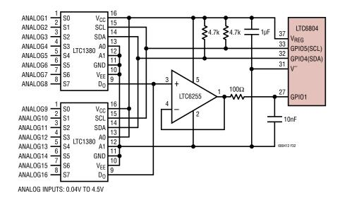
Figure 32. MUX Circuit Supports Sixteen Additional Analog Measurements
