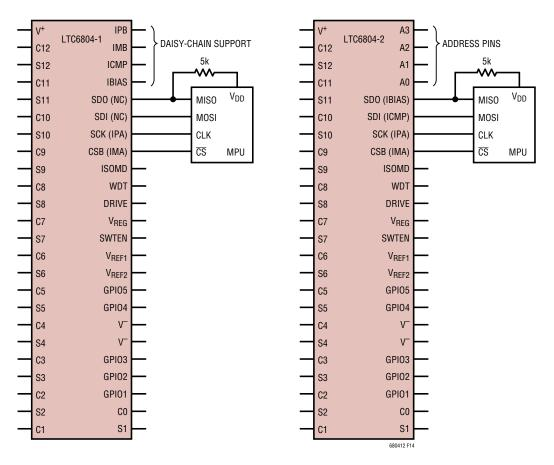
Figure 14. 4-Wire SPI Configuration
