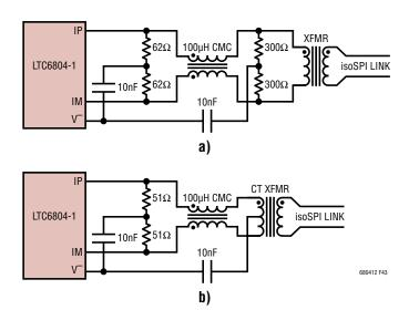
Figure 43. Daisy Chain Interface Components
