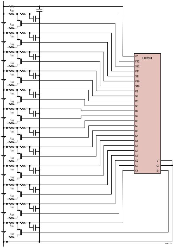
Figure 37. Balancing Self Test Circuit
