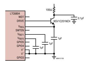
Figure 28. Simple V<sub>REG</sub> Power Source Using NPN Pass Transistor
