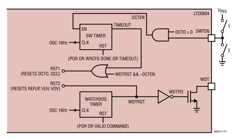
Figure 10. Watchdog and Software Discharge Timer
