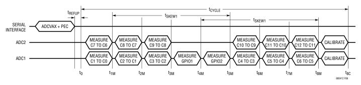
Figure 6. Timing of ADCVAX Command
