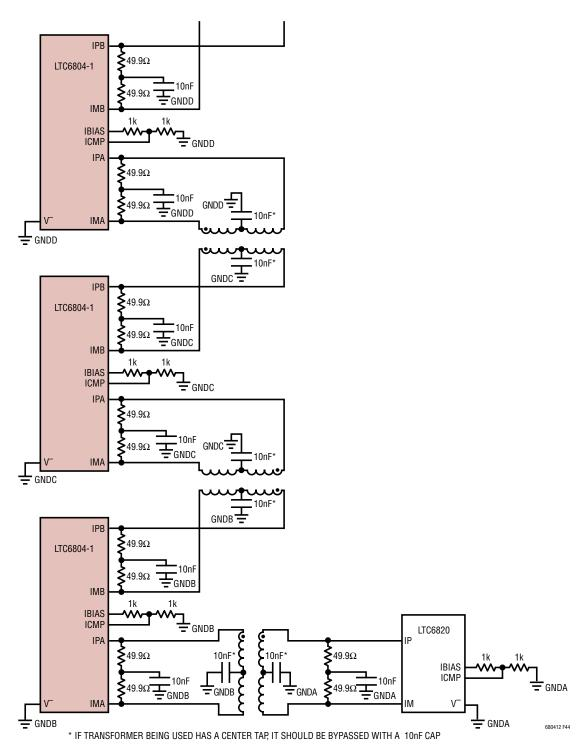
Figure 44. Daisy Chain Interface Components on Single Board
