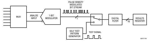
Figure 8. Operation of LTC6804 ADC Self Test
