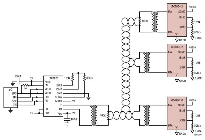
Figure 47. Connecting the LTC6804-2 in a Multi-Drop Configuration
