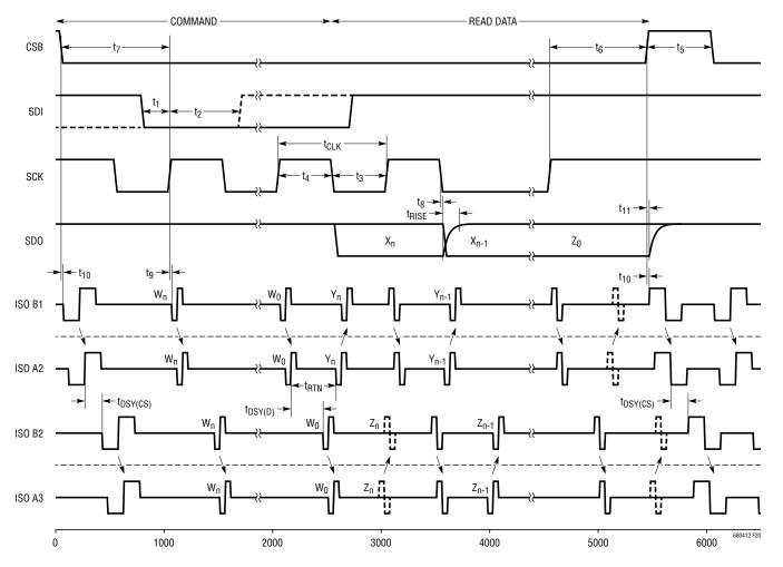
Figure 20. isoSPI Timing Diagram
