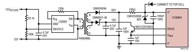
Figure 30. Powering LTC6804 from a Remote 12V Source
