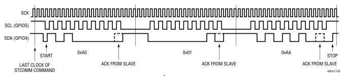
Figure 26. LTC6804 I<sup>2</sup>C Communication Example
