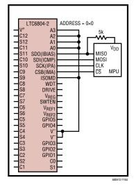
Figure 18d. Single-Device LTC6804-2 Using 4-Wire Port A
