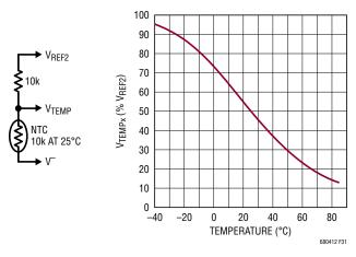
Figure 31. Typical Temperature Probe Circuit and Relative Output
