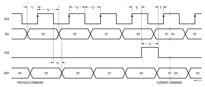
Figure 15. Timing Diagram of 4-Wire Serial Peripheral Interface
