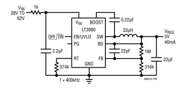
Figure 29. V<sub>REG</sub> Powered from Cell Stack with High Efficiency
