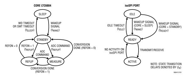
Figure 1. LTC6804 Operation State Diagram
