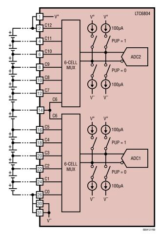
Figure 9. Open-Wire Detection Circuitry
