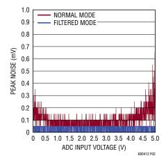
Figure 2. Measurement Noise vs Input Voltage
