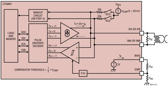
Figure 16. isoSPI Interface
