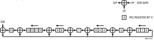
Figure 22. 15-Bit PEC Computation Circuit
