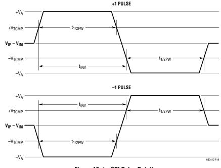
Figure 19. isoSPI Pulse Detail
