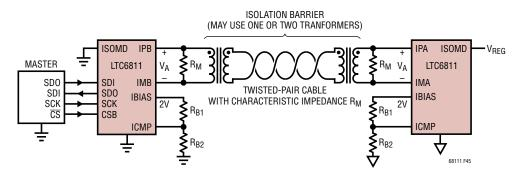
Figure 45. isoSPI Circuit
