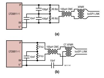
Figure 47. Daisy Chain Interface Components
