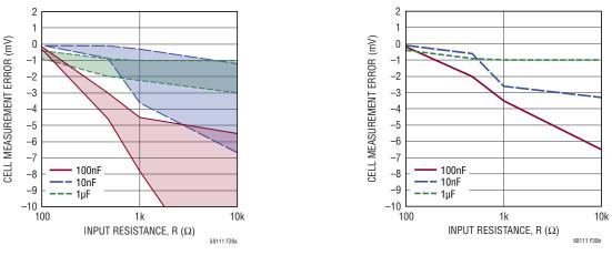
(a) Cell Measurement Error Range vs Input RC Values (b) Cell Measurement Error vs Input RC Values (Extra Conversion and Delay Before Measurement)
