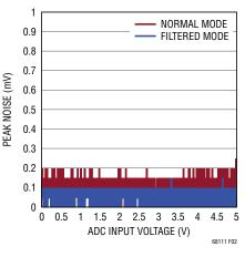
Figure 2. Measurement Noise vs Input Voltage
