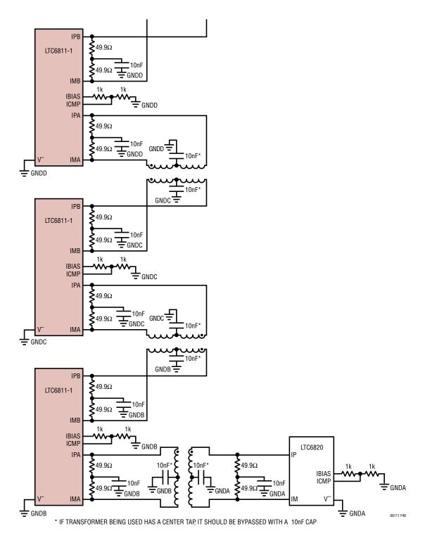
Figure 48. Daisy Chain Interface Components on Single Board
