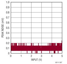
Measurement Error vs Input, **Filtered Mode**
