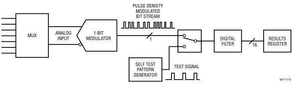
Figure 10. Operation of LTC6811 ADC Self Test
