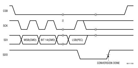
Figure 29. SDO Polling Using PLADC Command (Parallel Configuration)
