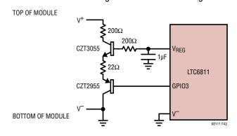
Figure 43. 200mA Module Balancer
