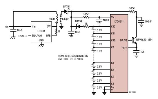
Figure 36. Flyback Converter to Power V<sup>+</sup> and V<sub>REG</sub>
