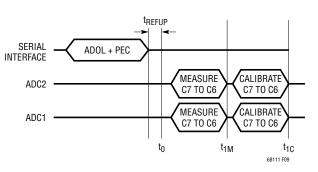
Figure 9. Timing for ADOL Command Measuring Cell 7 with both ADC1 and ADC2
