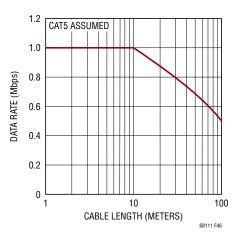
Figure 46. Data Rate vs Cable Length
