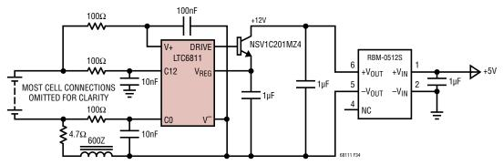
Figure 34. DC/DC Converter Module to Power  $V_{\text{REG}}$
