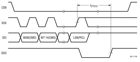
Figure 28. SDO Polling After an ADC Conversion Command (Parallel Configuration)
