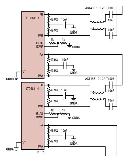
Figure 49. Capacitive Isolation Coupling for LTC6811-1s on the Same PCB
