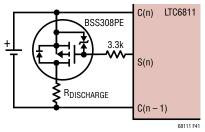
b) External Discharge Circuit
