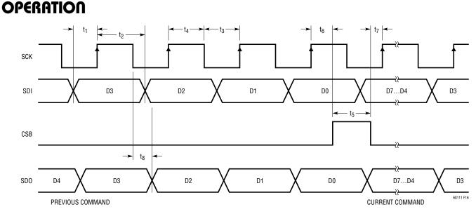
Figure 16. Timing Diagram of 4-Wire Serial Peripheral Interface
