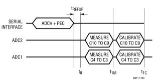
Figure 4. Timing for ADCV Command Measuring 2 Cells
