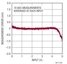
Measurement Noise vs Input, Normal Mode
