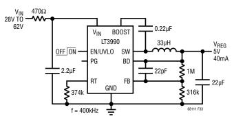
Figure 33.  $V_{\text{REG}}$  Powered From Cell Stack with High Efficiency Regulator
