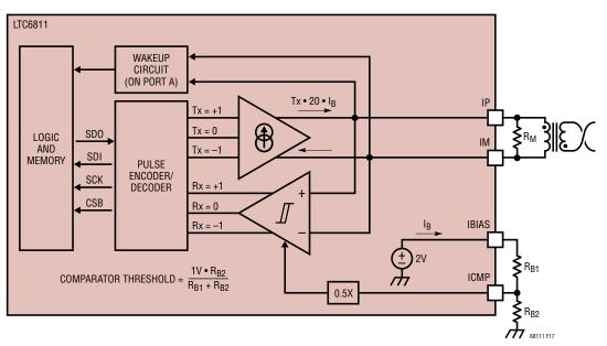
Figure 17. isoSPI Interface
