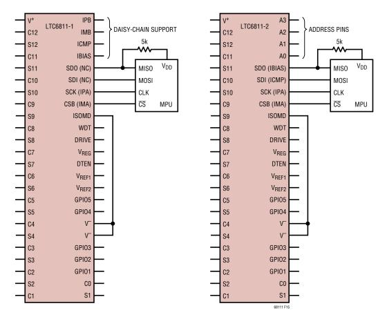
Figure 15. 4-Wire SPI Configuration
