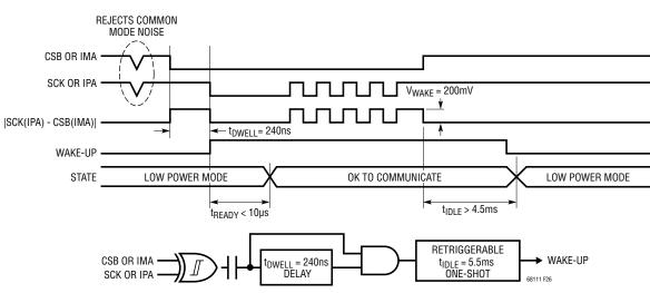
Figure 26. Wake-Up Detection and IDLE Timer
