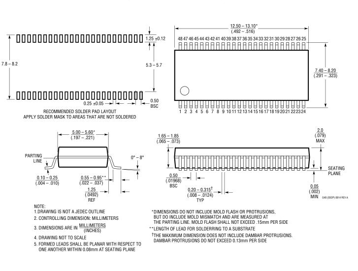
G Package 48-Lead Plastic SSOP (5.3mm) (Reference LTC DWG # 05-08-1887 Rev A)
