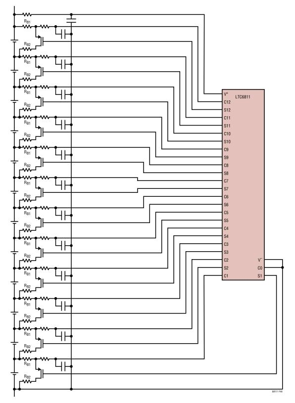
Figure 44. Balancing Self Test Circuit
