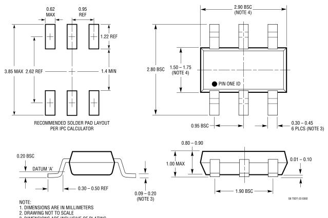
3. DIMENSIONS ARE INCLUSIVE OF PLATING 4. DIMENSIONS ARE EXCLUSIVE OF MOLD FLASH AND METAL BURR
