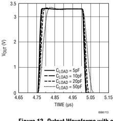
Figure 13. Output Waveforms with an Inductive Supply (See Figure 12)
