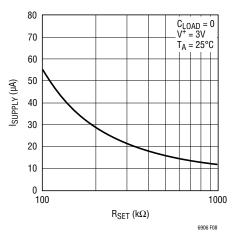
Figure 8. Unloaded Supply Current vs R<sub>SET</sub>
