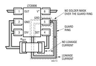
Figure 10. PC Board Layout with Guard Ring
