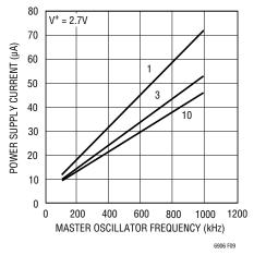
Figure 9. Supply Current vs Frequency
