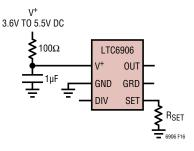
Figure 16. Using the LTC6906 at Higher Supply Voltages
