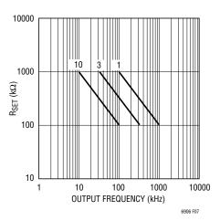
Figure 7. R<sub>SET</sub> vs Desired Output Frequency (LTC6906)
