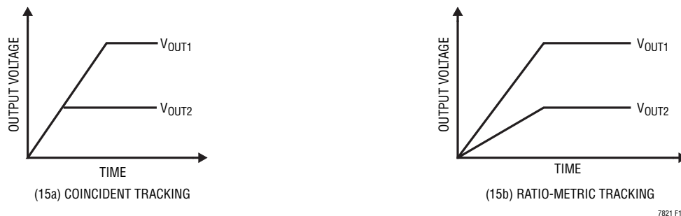
Figure 15. Two Different Methods of Output Voltage Tracking
