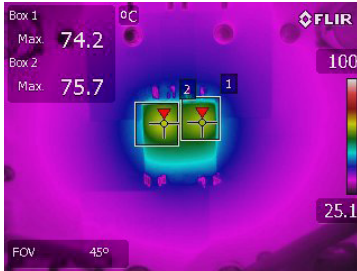
Figure 10. Thermal Image 12V to 1.0V, 36A with 200LFM without Heat Sink
