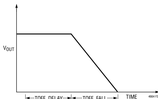
Figure 30. TOFF_DELAY and TOFF_FALL
