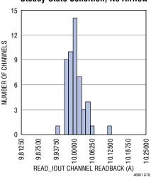
READ\_IOUT of 25 LTM4686s (DC2722) 12 $V_{IN}$ , 1 $V_{OUT}$ ,  $T_J = 125^{\circ}$ C,  $I_{OUT,n} = 10$ A, System Having Reached Thermally Steady-State Condition, No Airflow
