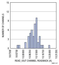
READ\_IOUT of 25 LTM4686s (DC2722) 12V<sub>IN</sub>, 1V<sub>OUT</sub>, T<sub>J</sub> = 25°C, I<sub>OUT</sub>, = 10A, System Having Reached Thermally Steady-State Condition, No Airflow
