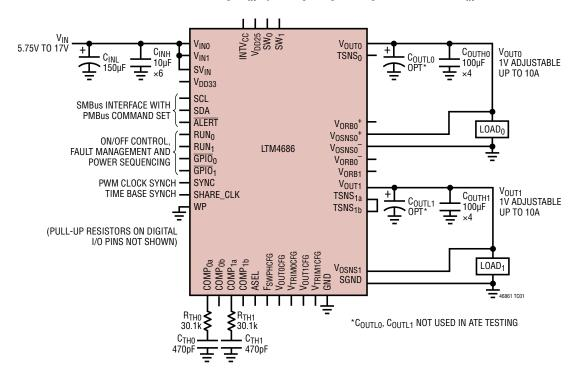
Test Circuit 2. LTM4686-1 ATE Low  $V_{\text{IN}}$  Operating Range Configuration,  $4.5\text{V} \leq V_{\text{IN}} \leq 5.75\text{V}$
