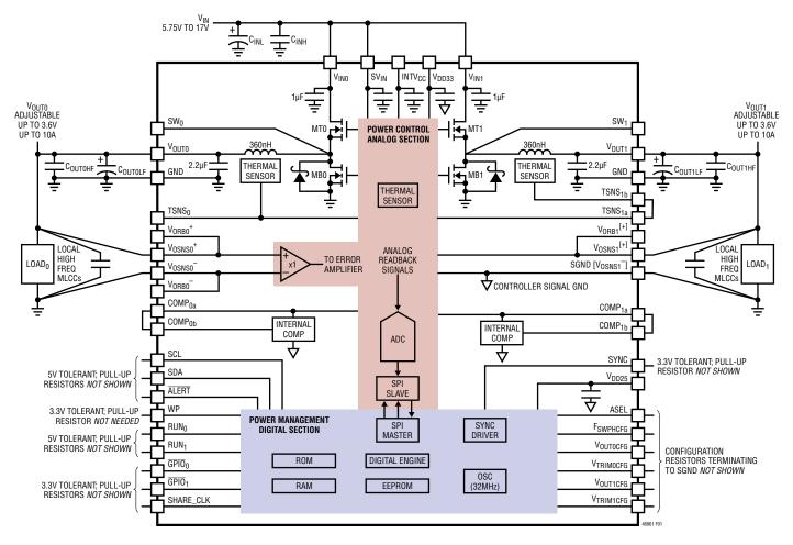
Figure 1. Simplified LTM4686 Block Diagram
