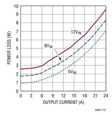
Figure 11. 1V<sub>OUT</sub> Power Loss Curve
