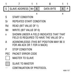
Figure 37. PMBus Packet Protocol Diagram Element Key
