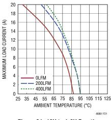
Figure 21. 12V to 1.8V Derating Curve, with Heat Sink
