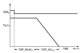
Figure 4. TOFF\_DELAY<sub>n</sub> and TOFF\_FALL<sub>n</sub>
