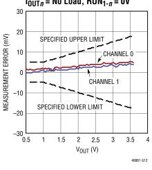
READ\_IOUT<sub>n</sub> (Output Current Readback) Error vs I<sub>OUTn</sub>
