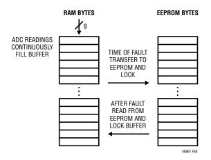
Figure 60. Fault Log Conceptual Diagram
