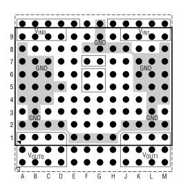
(b) PCB Layout to Accommodate Any of LTM4686 or LTM4675 or LTM4676A or LTM4677 Modules
