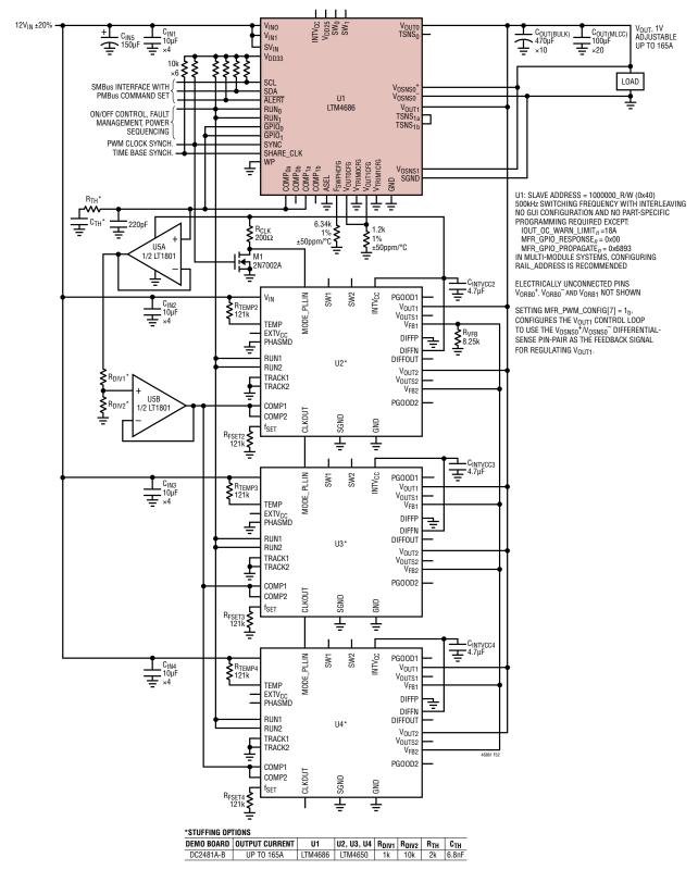
Figure 32. One LTM4686 Operating In Parallel with 3xLTM4650 (See Demo Board DC2481A-B, Custom-Stuffed with LTM4686 Module for U1) Producing 1V<sub>OUT</sub> at up to 165A. Power System Management Features Accessible Through LTM4686. See Figure 33. Contact Sales Support for Adapting Circuit for LTM4686 Use with LTM4631, LTM4620A, LTM4630
