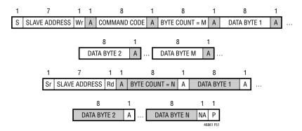
Figure 51. Block Write – Block Read Process Call
