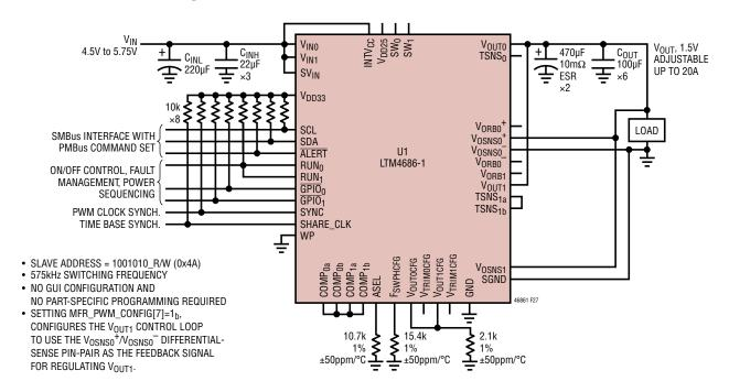
Figure 27. 20A, 1.5V Output DC/DC μModule Regulator with I<sup>2</sup>C/SMBus/PMBus Serial Interface
