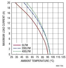
(35b)  $12V_{IN}$ , with Table 18 Heat Sink
