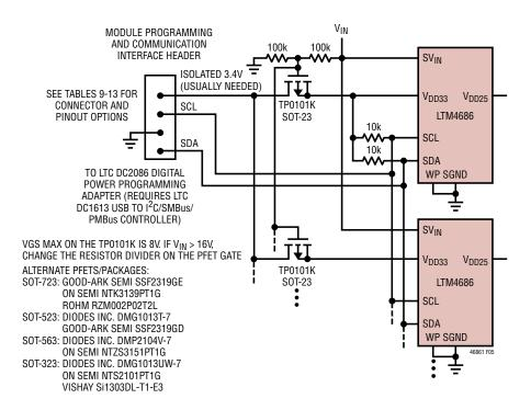
Figure 5. Circuit Suitable for Programming EEPROM/NVM of LTM4686 and Other ADI PSM Modules/ICs in Vast Systems, Even When  $V_{IN}$  Power is Absent,  $0^{\circ}C < T_{.I} \le 85^{\circ}C$
