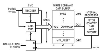
Figure 8. Write Command Data Processing
