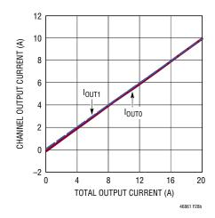
(28b) 12V $_{\rm IN}$ , Figure 27 Circuit with U1 Installed with LTM4686, INTV $_{\rm CC}$  Open and V $_{\rm OUT}$  Commanded to 1V
