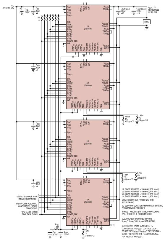
Figure 31. Four Paralleled LTM4686 Producing  $1V_{OUT}$  at Up to 78A. Integrated Power System Management Features Accessible Over 2-Wire  $I^2C/SMBus/PMBus$  Serial Interface. Evaluated on DC1989B-C, Custom-Stuffed with LTM4686 Modules
