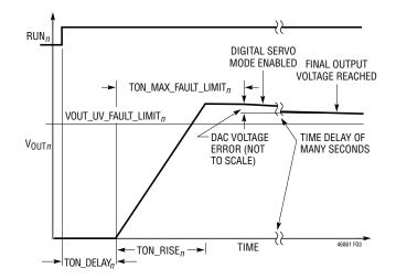
Figure 3. Timing Controlled Vout Rise
