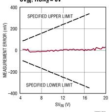
MFR\_READ\_IIN $_n$  (Input Current Readback) Error vs ( $I_{VIN}n + I_{SVIN}$ ), MFR\_PWM\_MODE $_n$ [0]=1 $_b$ ,  $I_{OUT}n$  Swept from 0A to 10A, One Channel at a Time, RUN $_{1-n}$  = 0V
