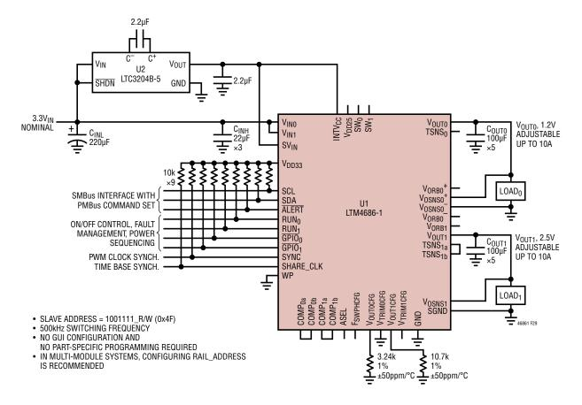
Figure 29. 10A, 1.2V and 2.5V Outputs Generated from 3.3V Power Input and Providing I<sup>2</sup>C/SMBus/PMBus Serial Interface
