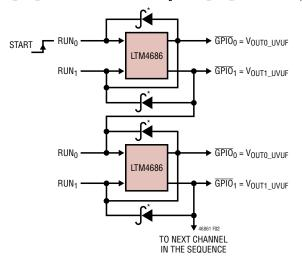
NOTE: RESISTOR OR RC PULL-UPS ON  $\text{RUN}_{\it{H}}$  and  $\overline{\text{GPIO}}_{\it{H}}$  pins not shown \*OPTIONAL SIGNAL SCHOTTKY DIODE. ONLY NEEDED WHEN ACCURATE PGOOD (POWER GOOD) INDICATION IS REQURED BY THE SYSTEM/USER IMMEDIATELY AT SVIN POWER UP
