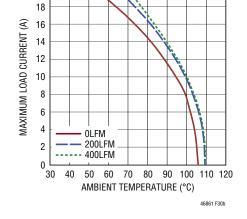
(30a) Single 20A, 1V<sub>OUT</sub>, No Heat Sink
