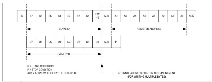
Figure 18. I<sup>2</sup>C Single Byte Write Transaction
