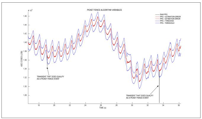
Figure 10. Picket Fences Variables In A PPG Waveform
