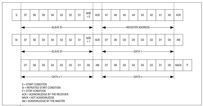
Figure 21. I<sup>2</sup>C Multi-Byte Read Transaction
