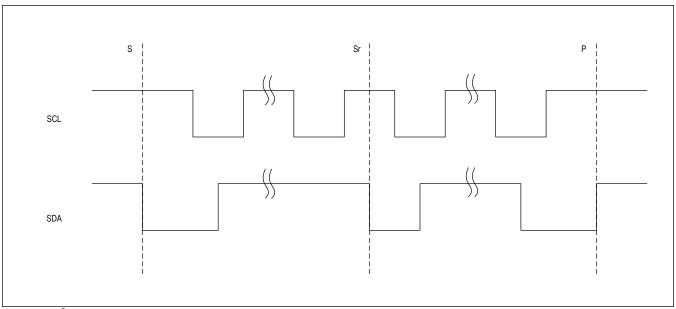
Figure 16. I<sup>2</sup>C START, STOP, and REPEATED START Conditions
