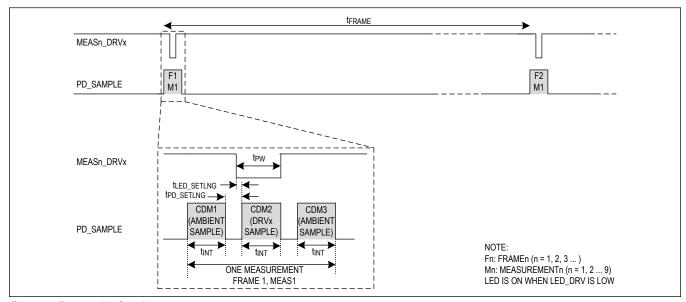
Figure 4. Frame with One Measurement
