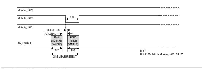
Figure 8. Forward Difference Method (FDM)
