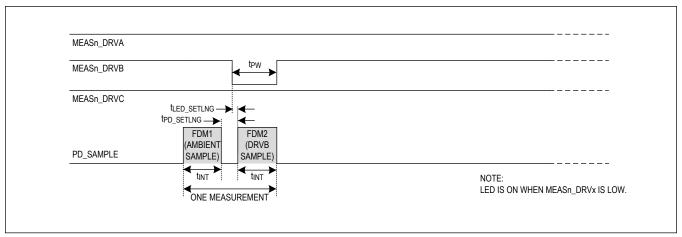
Figure 3. Measurement with FDM
