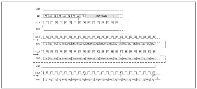
Figure 14. SPI FIFO Burst Mode Read Transaction
