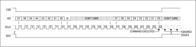
Figure 12. SPI Write Transaction
