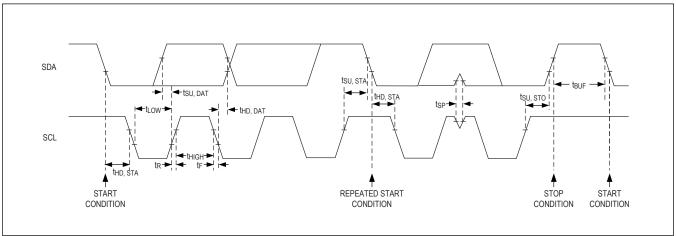
Figure 15. Detailed I<sup>2</sup>C Timing Diagram
