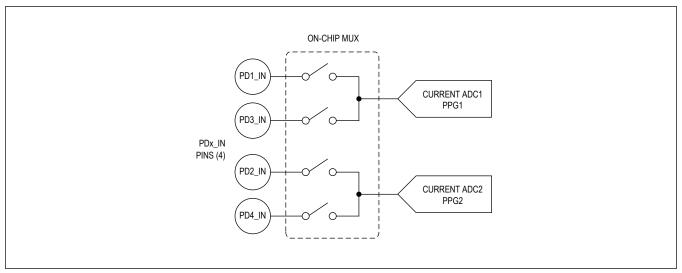
Figure 1. On-Chip Mux for the PDx\_IN Pins
