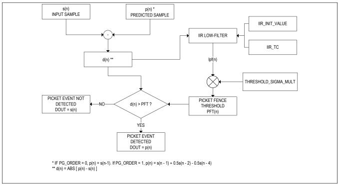
Figure 9. Picket Fence Function Flow
