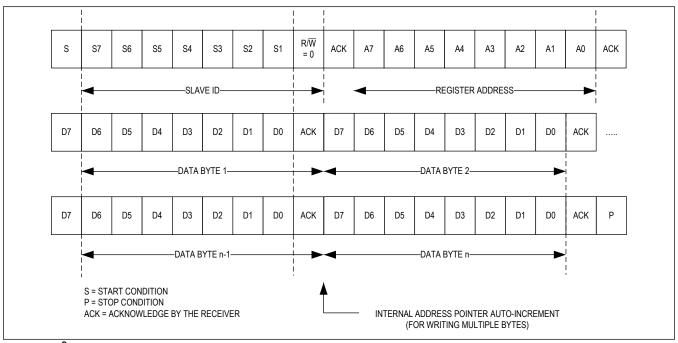
Figure 19. I<sup>2</sup>C Multi-Byte Write Transaction
