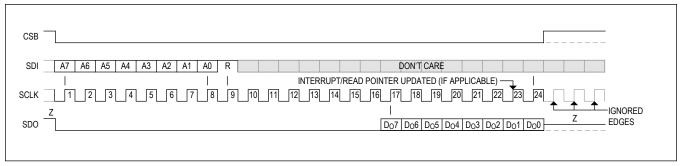
Figure 13. SPI Read Transaction
