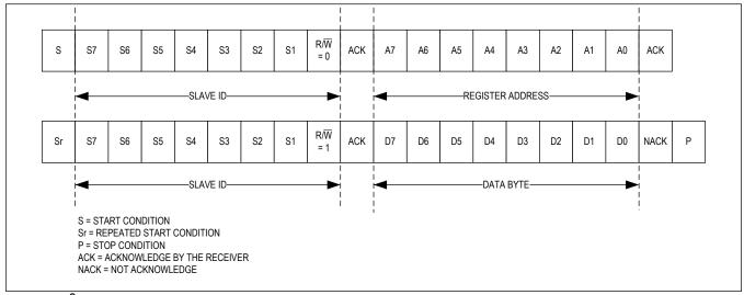
Figure 20. I<sup>2</sup>C Single Byte Read Transaction
