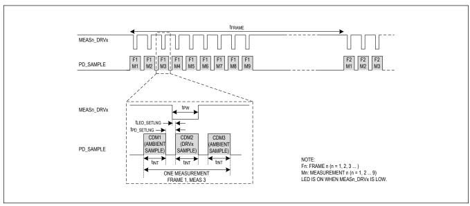
Figure 5. Frame with Nine Measurements
