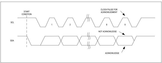
Figure 17. I<sup>2</sup>C Acknowledge Bit
