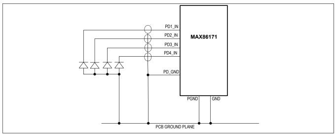
Figure 22. PCB Layout Recommendation
