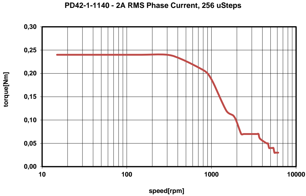
Figure 9.1 PD42-1-1140 torque vs. velocity 24V / 2A, 256µsteps
