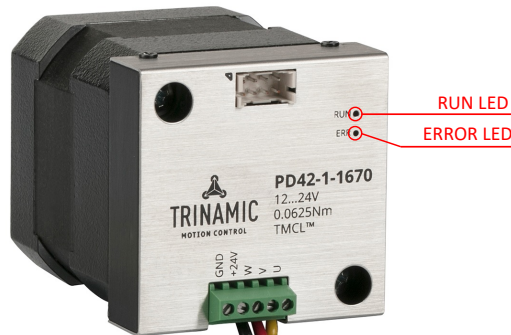
Figure 5: PD-x-1670 LED location
