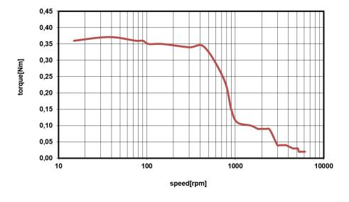
Figure 15: PD42-2-1240 torque vs. velocity 24V / 2A, 256μsteps
