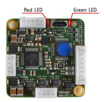
Figure 3: PD42-x-1240 LEDs
