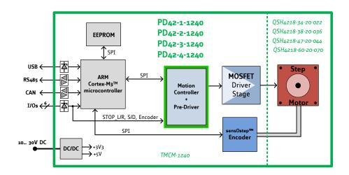
Figure 18: PD42-x-1240 block diagram
