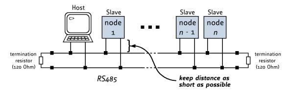
Figure 10: RS485 bus structure with termination resistors
