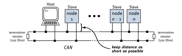
Figure 13: CAN bus structure with termination resistors
