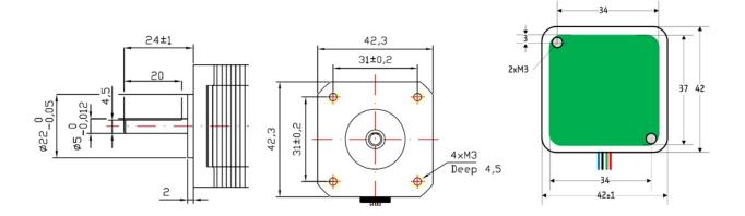
Figure 1: PD42-x-1240 with different NEMA17 / 42mm stepper motors (all dimensions in mm)
