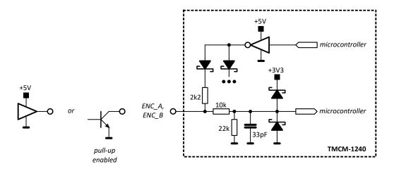
Figure 8: External encoder input
