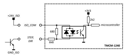
Figure 9: Step/Direction input
