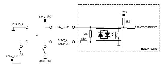
Figure 7: Stop switch inputs
