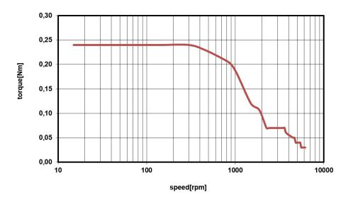
Figure 14: PD42-1-1240 torque vs. velocity 24V / 2A, 256μsteps
