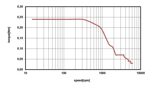
Figure 9: PD42-1-1370 torque vs. velocity 24V / 2A, 256µsteps, open-loop
