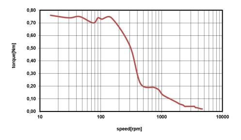
Figure 12: PD42-4-1370 torque vs. velocity 24V / 2A, 256µsteps, open-loop
