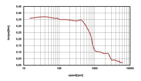
Figure 10: PD42-2-1370 torque vs. velocity 24V / 2A, 256µsteps, open-loop
