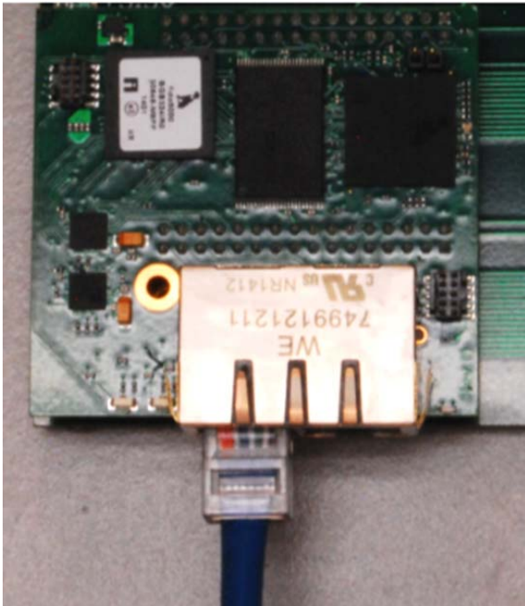
Figure 6. Ethernet Cable Connection
