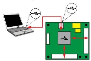
Figure 3. SDP-B controller functional overview.
