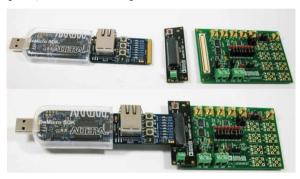
Figure 6. BeMicro SDK, interposer, and SDP controller.
