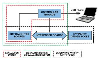
Figure 1. System Demonstration Platform overview.
