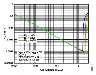
Figure 10. THD + N vs. Amplitude,  $V_{SY} = \pm 5 V$
