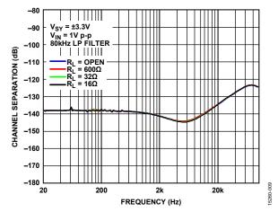
Figure 9. Channel Separation vs. Frequency,  $V_{SY} = \pm 3.3 \text{ V}$
