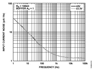
Figure 19. Input Current Noise vs. Frequency
