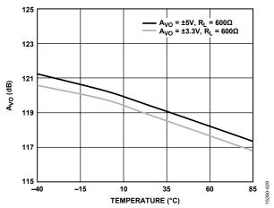
Figure 29. Open-Loop Gain (Avo) vs. Temperature
