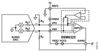
Figure 42. Common-Mode Circuit with Common-Mode Control
