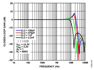
Figure 45. Frequency Response for Driving Capacitive Loads,  $V_{SY} = \pm 3.3 \text{ V}$
