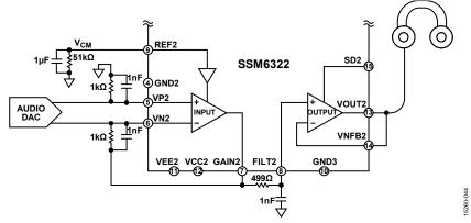
Figure 46. SSM6322 Circuit with Current Output DAC
