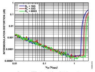
Figure 16. CCIF vs. Input Voltage ( $V_{IN}$ ),  $V_{SY} = \pm 5 V$
