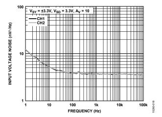
Figure 18. Input Voltage Noise vs. Frequency,  $V_{SY} = \pm 3.3 \text{ V}$
