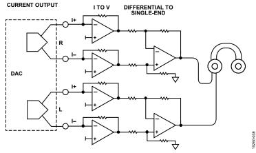
Figure 41. Current Output DAC Configuration
