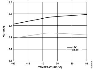
Figure 36. Supply Current  $(+I_{SY})$  vs. Temperature
