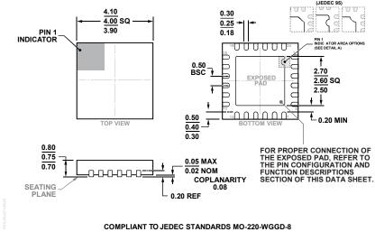
Figure 49. 24-Lead Lead Frame Chip Scale Package [LFCSP] 4 mm × 4 mm Body and 0.75 mm Package Height (CP-24-15) Dimensions shown in millimeters
