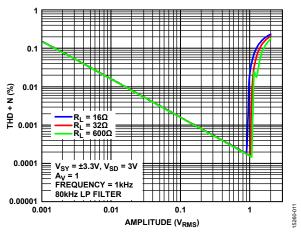
Figure 11. THD + N vs. Amplitude,  $V_{SY} = \pm 3.3 \text{ V}$
