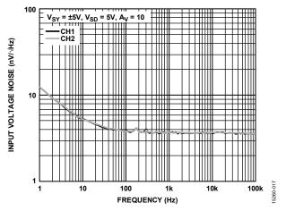
Figure 17. Input Voltage Noise vs. Frequency,  $V_{SY} = \pm 5 V$
