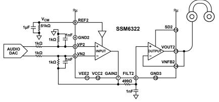
Figure 47. SSM6322 Circuit with Voltage Output DAC
