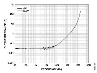
Figure 20. Enabled Output Impedance vs. Frequency
