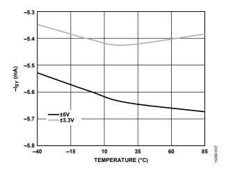
Figure 37. Supply Current (–I<sub>SY</sub>) vs. Temperature
