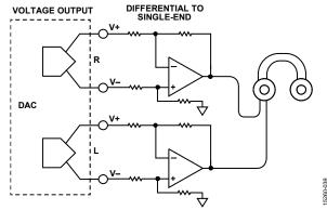
Figure 39. Voltage Output DAC Configuration
