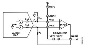
Figure 40. Common-Mode Circuit Without Common-Mode Control
