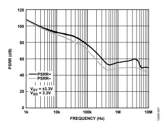
Figure 7. PSRR vs. Frequency,  $V_{SY} = \pm 3.3 \text{ V}$
