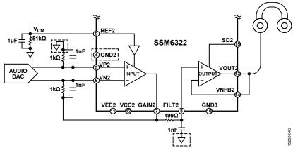
Figure 48. Sensing Ground of Input Stage
