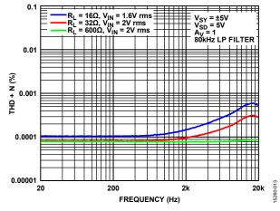
Figure 13. THD + N vs. Frequency,  $V_{SY} = \pm 5 V$
