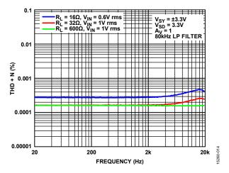
Figure 14. THD + N vs. Frequency,  $V_{SY} = \pm 3.3 \text{ V}$
