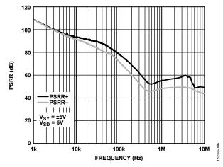
Figure 6. PSRR vs. Frequency,  $V_{SY} = \pm 5 V$
