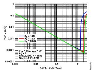
Figure 12. THD + N vs. Amplitude,  $V_{SY} = \pm 6 V$
