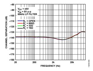
Figure 8. Channel Separation vs. Frequency,  $V_{SY} = \pm 5 V$
