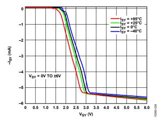
Figure 28. Supply Current (-Isy) vs. Supply Voltage (Vsy)
