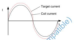
Coil current does not have optimum shape
