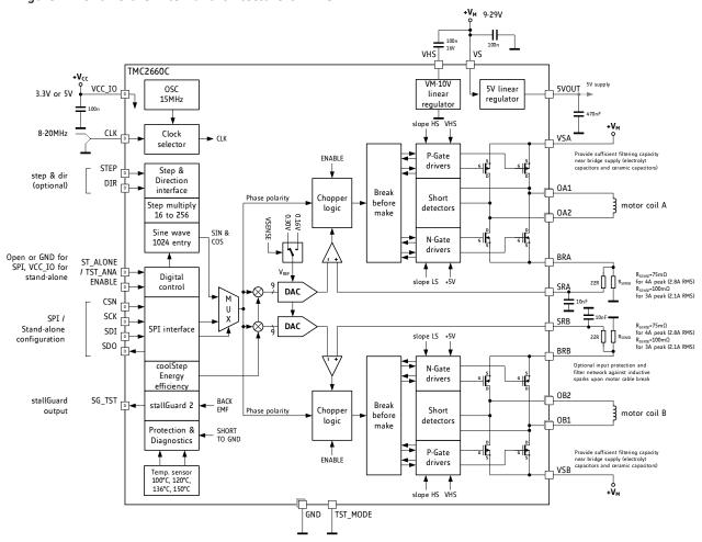
Figure 3.1 TMC2660 block diagram
