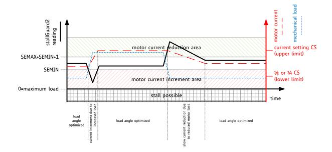
Figure 6.2 CoolStep adapts motor current to the load.
