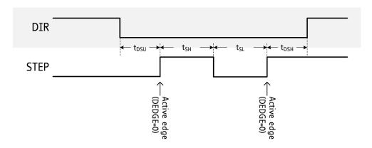
Figure 8.1 STEP and DIR timing.
