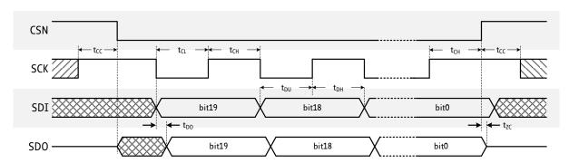
Figure 7.1 SPI Timing
