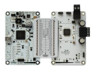
Evaluation board system with TMC2660
