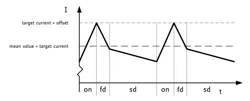
Figure 10.4 Constant off-time chopper with offset showing the coil current during two cycles
