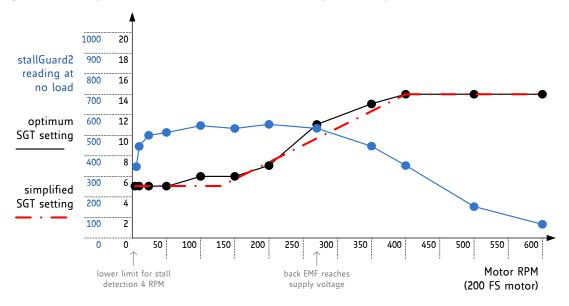
Figure 5.2 Linear interpolation for optimizing SGT with changes in velocity.
