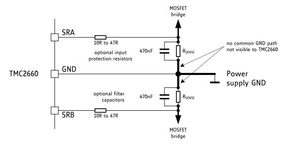
Figure 9.1 Sense resistor grounding and protection components
