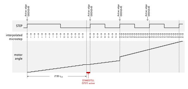
Figure 8.3 MicroPlyer microstep interpolation with rising STEP frequency.
