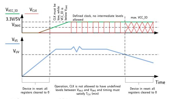
Figure 14.1 Start-up requirements of CLK input
