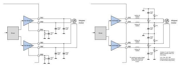
Figure 16.1 Simple ESD enhancement and more elaborate motor output protection
