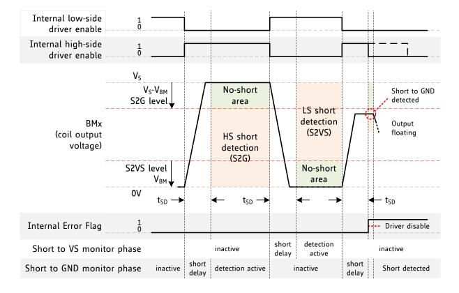
Figure 12.1 Short detection timing
