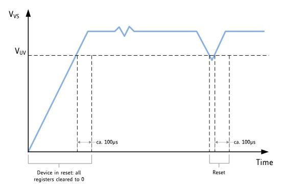
Figure 12.2 Undervoltage reset timing
