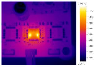
Figure 19.1 TMC2660 operating at 2.3A RMS (3.2A peak) on a 50cm<sup>2</sup> sized board
