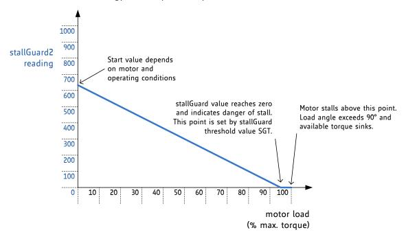
Figure 5.1 StallGuard2 load measurement SG as a function of load
