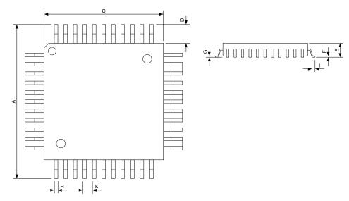
Figure 20.1 Dimensional drawings (PQFP44)
