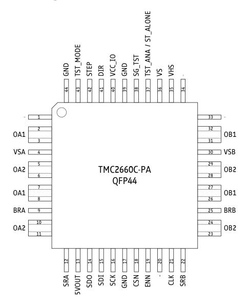
Figure 2.1 TMC2660 pin assignment (top view)
