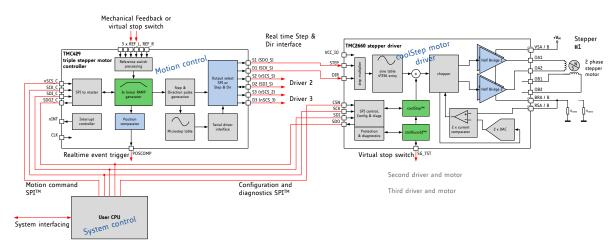
Figure 7.2 Interfaces to a TMC429 motion controller chip and a TMC2660 motor driver
