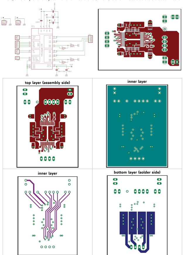
Figure 17.1 Layout example for TMC2660
