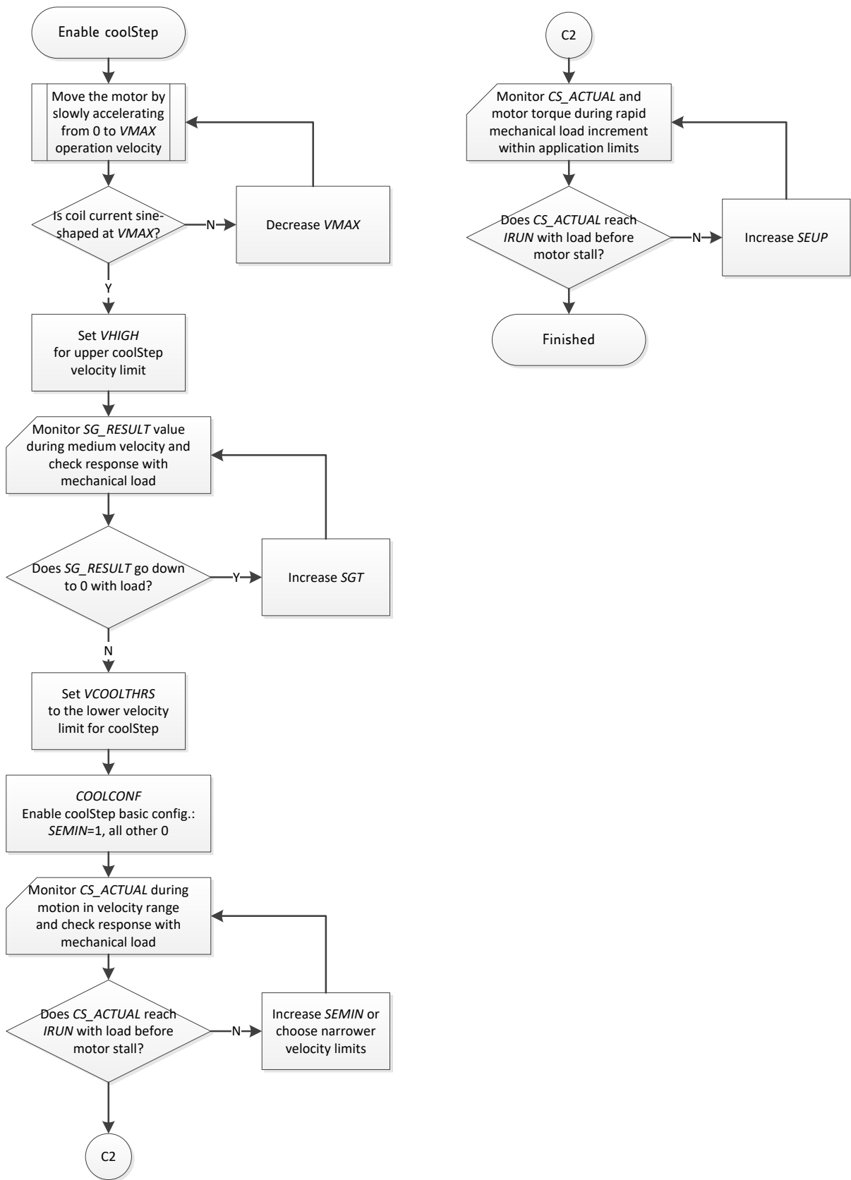
Figure 14.4 Enabling coolStep (only in combination with spreadCycle)
