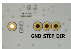
Figure 3.3 Test points for GND, REFL_STEP, and REFR_DIR
