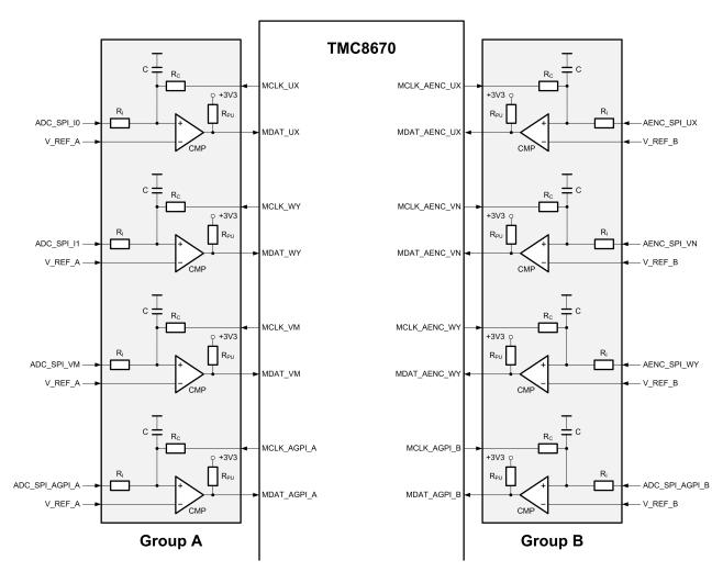
Figure 15: TMC8670 Delta Sigma ADC Configuration
