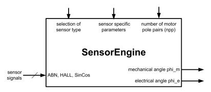
Figure 2: TMC8670 Sensor Engine maps position sensor signals to mechanical angels and electrical angels as direct input for the FOC engine.
