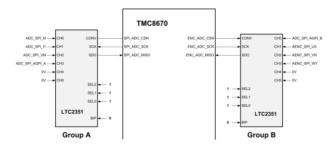
Figure 16: TMC8670 configuration for LTC2351 SPI ADCs
