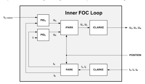
Figure 28: Inner FOC Control Loop
