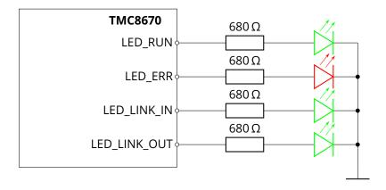
Figure 8: Status LED circuit
