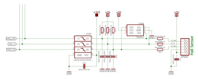
Figure 13: Example circuit for connecting Hall sensor signals with level shifters from typically 5V to 3.3V
