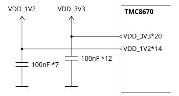
Figure 7: PLL supply filter
