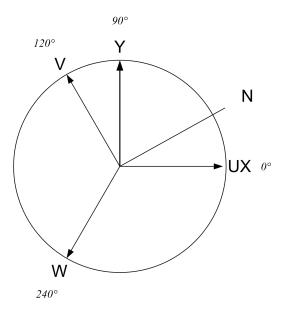
Figure 11: ABN Incremental Encoder N Pulse
