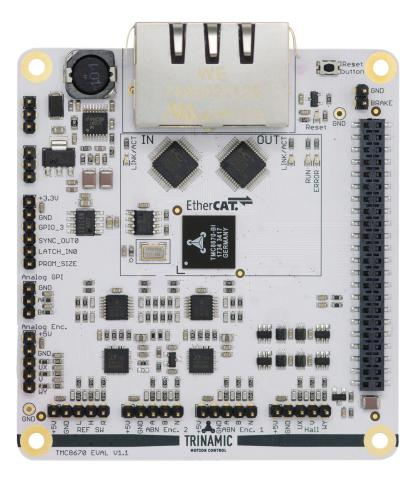
Figure 3: TMC8670 Evaluation Board
