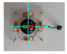
Figure 25: Compass Motor Model w/ 3 Phases UVW (FOC3) and Compass Motor Model w/ 2 Phases (FOC2)
