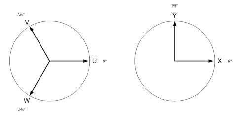
Figure 24: Orientations UVW (FOC3) and XY (FOC2)
