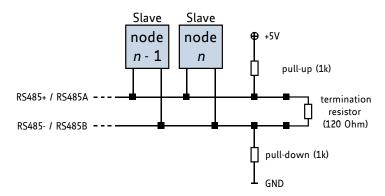
Figure 3.5 Bus lines with resistor network
