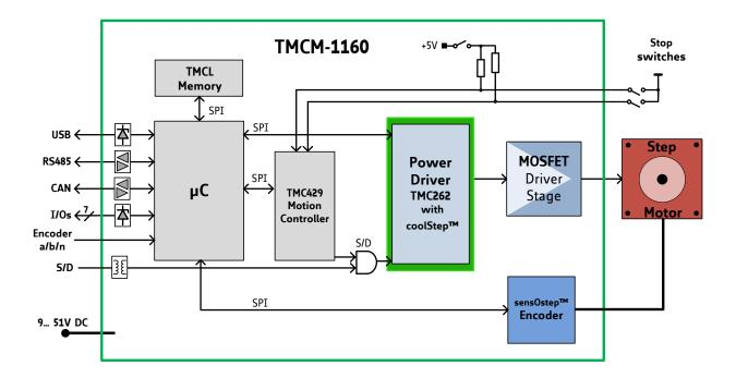
Figure 8.1 Main parts of the TMCM-1160
