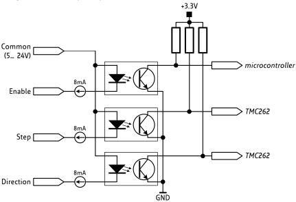
Figure 3.9 Step / Direction / Enable inputs
