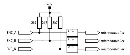
Figure 3.9 Encoder a/b/n inputs
