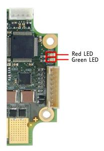
Figure 6.1 On-board LEDs
