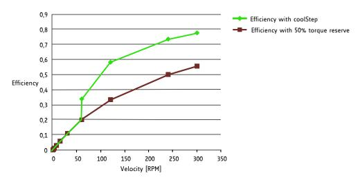
Figure 1.2 Energy efficiency example with coolStep
