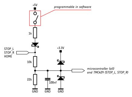
Figure 3.6 STOP\_L, STOP\_R and HOME inputs (simplified input circuit)
