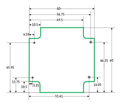
Figure 3.1 Dimensions and mounting holes
