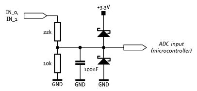
Figure 3.7 General purpose inputs (simplified input circuit)
