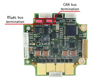
Figure 4.1 RS485 and CAN bus termination
