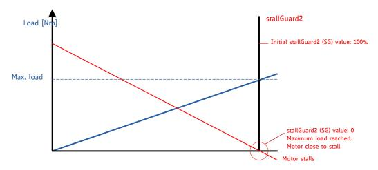
Figure 3: stallGuard2 Load Measurement as a Function of Load
