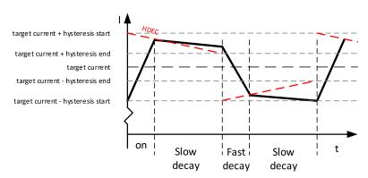
Figure 2: spreadCycle principle
