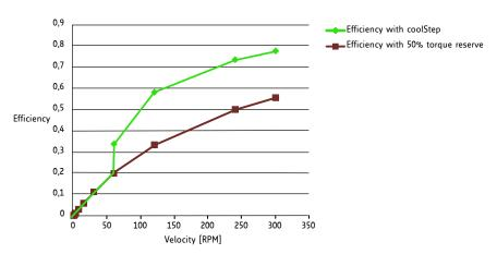
Figure 4: Energy Efficiency Example with coolStep
