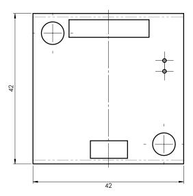
Figure 6: TMCM-1270 top view mechanical dimensions
