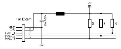
Figure 4.3: Hall sensor input circuit
