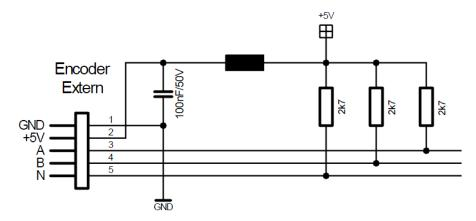
Figure 4.4: Encoder input circuit
