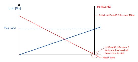
Figure 1: StallGuard2 Load Measurement as a Function of Load
