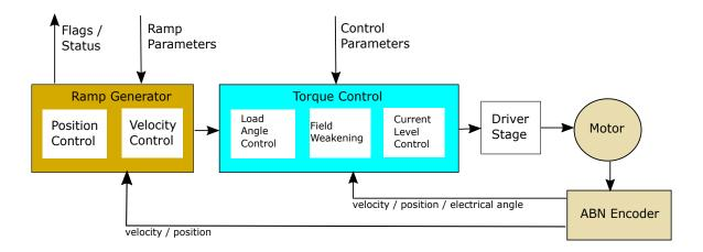
Figure 11: Closed-Loop Control Scheme
