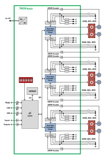
Figure 10.1 Main parts of the TMCM-6210
