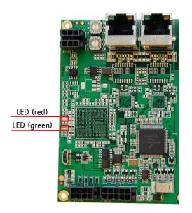
Figure 7.2: LEDs on TMCM-6210 interface brick
