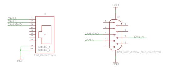
Figure 5.7: RJ45-2-DSUB schematic / connector pin assignment
