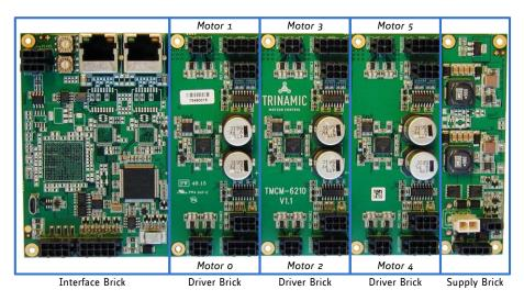
Figure 5.1 different bricks used for the TMCM-6210 / TMCM-6211
