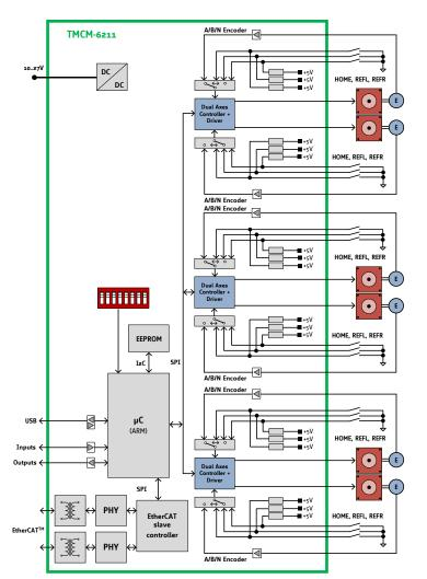
Figure 11.1 Main parts of the TMCM-6211
