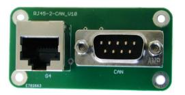
Figure 5.6: RJ45-2-DSUB PCB top view
