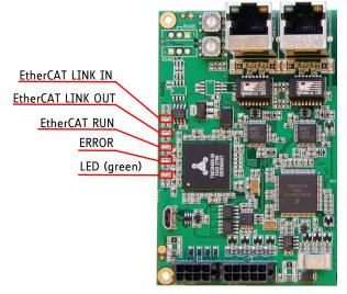
Figure 7.3: LEDs on TMCM-6211 interface brick
