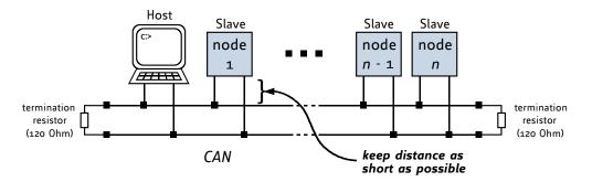
Figure 5.6: CAN bus structure
