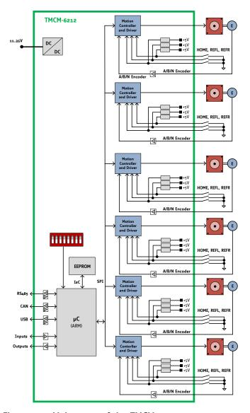
Figure 10.1 Main parts of the TMCM-6212
