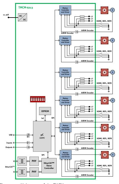
Figure 11.1 Main parts of the TMCM-6213
