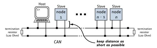
Figure 5.6: CAN bus structure
