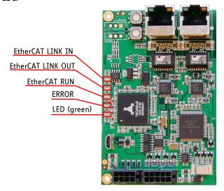
Figure 7.3: LEDs on TMCM-6213 interface brick
