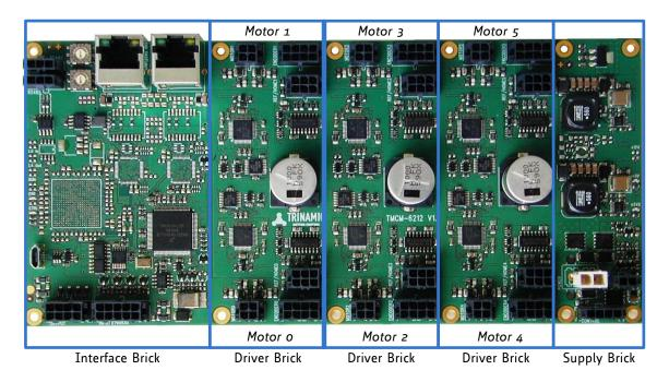
Figure 5.1 different bricks used for the TMCM-6212 / TMCM-6213
