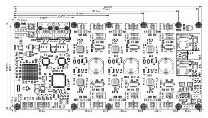
Figure 4.1 Dimension of TMCM-6212 / TMCM-6213 and position of mounting holes
