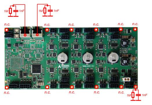
Figure 4.2 TMCM-6212 / TMCM-6213 mounting hole connections
