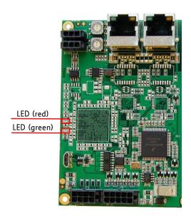
Figure 7.2: LEDs on TMCM-6212 interface brick
