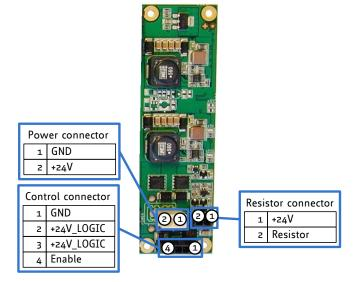
Figure 5.5: TMCM-6212 + TMCM-6213 Power supply Brick
