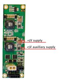
Figure 7.1: LEDs on power supply brick
