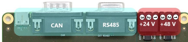
Figure 3: Power; Communication and USB-C connectors of TMCM-BB1
