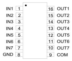
DIP-16/SOP-16/TSSOP-16 (Top View)
