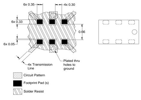
Dimensions are in Millimeters Mounting Footprint
